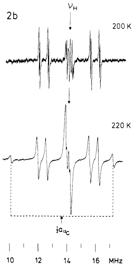
Figure 5. ENDOR spectra taken from ^{13}\text{C} biphenyl galvinoxyl 2b at different experimental conditions: (top) 200 K, B_{\text{NMR}} = 2.7G_{\text{rot}} , (bottom) 220 K, B_{\text{NMR}} = 6.2G_{\text{rot}} .
