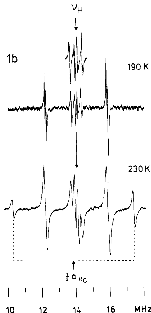
Figure 4. ENDOR spectra taken from ^{13}\text{C} phenylgalvinoxyl 1b at different experimental conditions; (top) 190 K, B_{\text{NMR}} = 2G_{\text{rot}} , for insert see text; (bottom) 230 K, B_{\text{NMR}} = 6.2G_{\text{rot}} .
